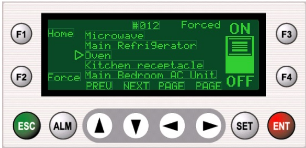
FIGURE 3.1 the force select screen consists of an ON/OFF switch object, scrolling, numerical and dynamic text fields and scrolling and navigation function keys.
