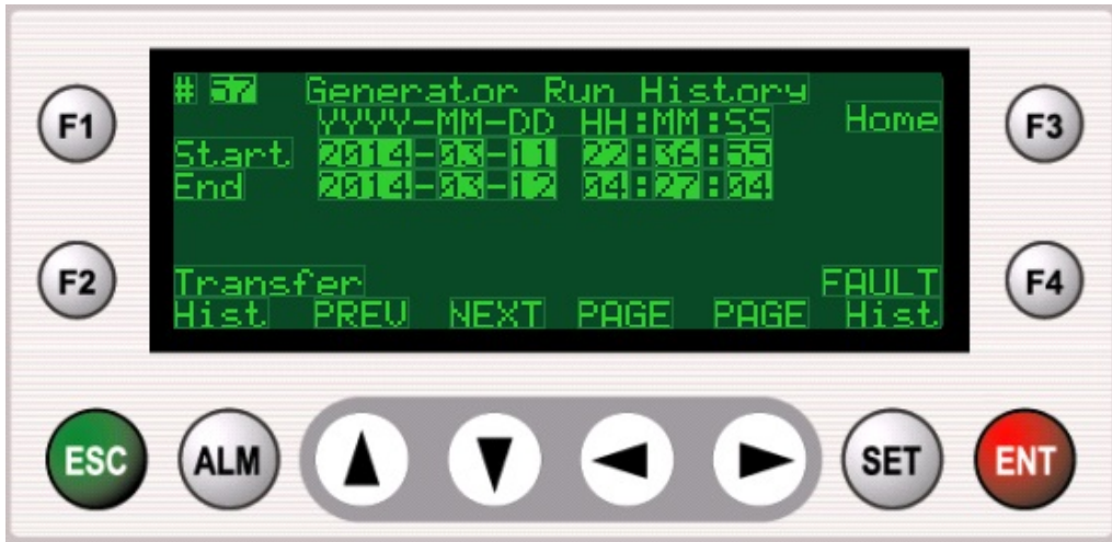
FIGURE 6.1 The Run History review screen consists of numerical fields and scrolling and navigation keys.
