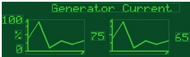
FIGURE 2.1 the main window consists of line trends and numerical displays, a rotation display and navigation function keys.
