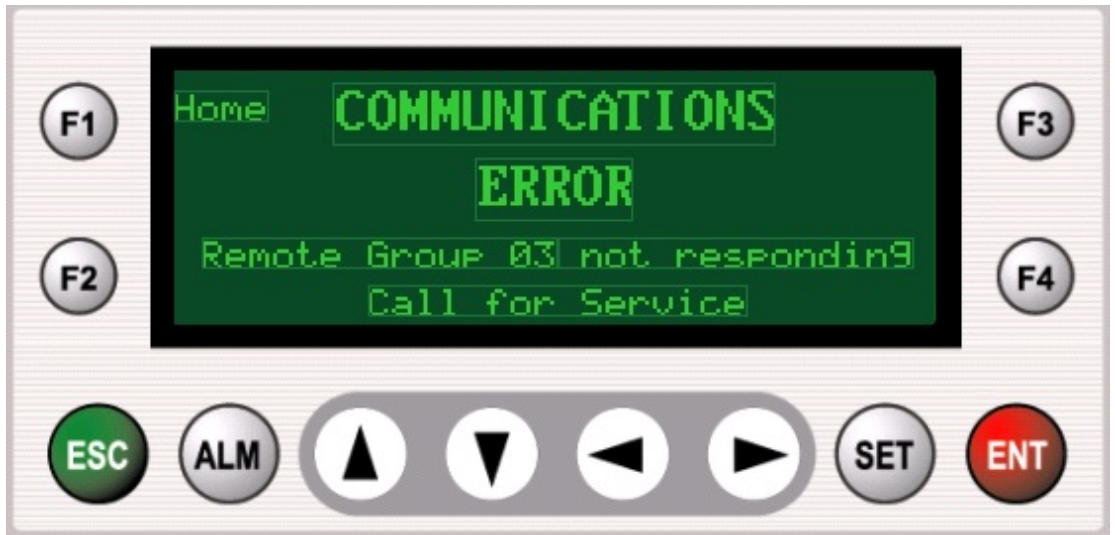
FIGURE 11.1 The Communications Error screen consists of text and numeric fields and a function key.
