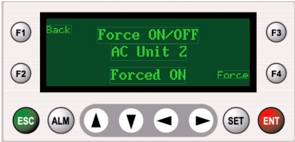
FIGURE 4.1 the force circuit screen consists of dynamic text fields and force and navigation function keys.
